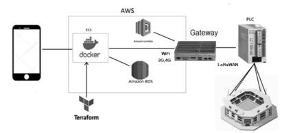
Fig. 1. Block diagram of a sports stadium lighting system based on the Internet of Things platform
