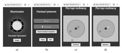
Fig. 6. Navigation of the user application «Illuminator» - a) the main screen of the application,b) the settings screen, c) the control screen of the lights, d) the event screen
