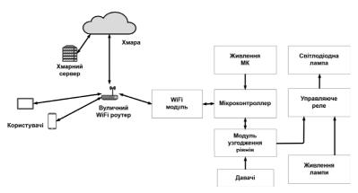
Fig. 1. Block diagram of the street lighting system
